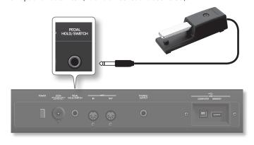
You can select the function that the footswitch should perform (p. 52). By default, the footswitch will control the "Hold" function.
