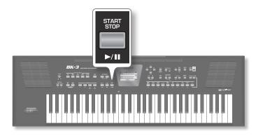
This button is used to start and stop rhythm playback. While a rhythm is running, the button's indicator flashes red on the first beat of each bar, and green on the remaining beats.
